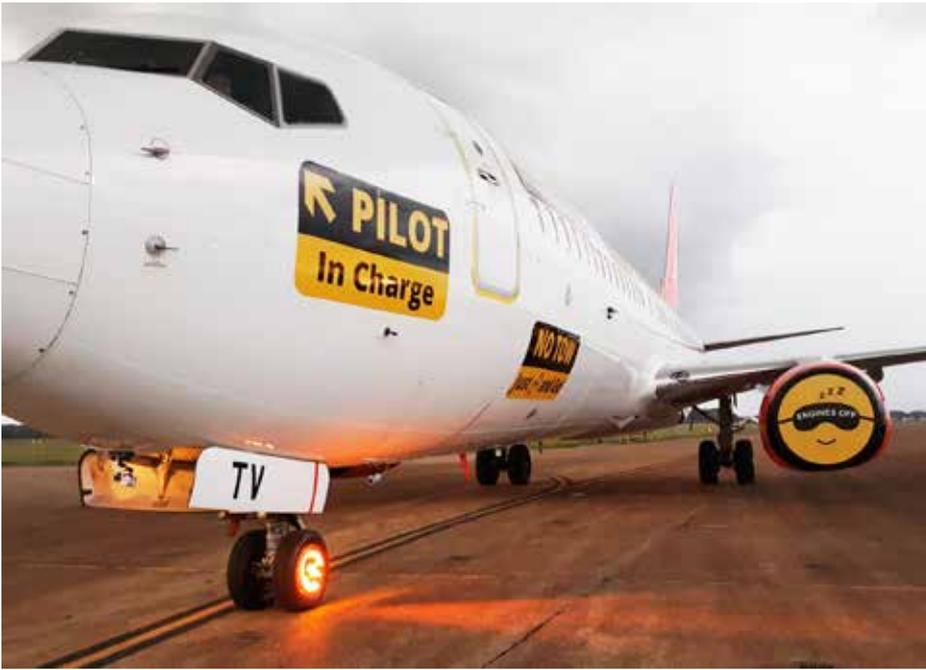
WheelTug has no impact on an aircraft’s airworthiness, Silvius insists, because the installation of the system does not require significant structural alterations to an aircraft, while any maintenance to WheelTug can be performed during an aircraft’s regular line maintenance schedule.
