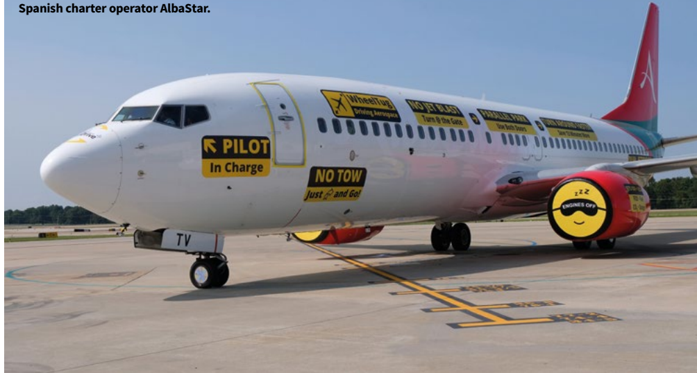
Getting off the ground: WheelTug has installed its system for trials with launch customer, Spanish charter operator AlbaStar.
